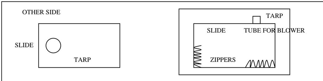
**TO DEFLATE:** Make sure everyone is out of slide, shut blower off, unplug blower from electrical outlet. Disconnect blower and open air release stub to deflate. Open zippers and roll it up once all air is out.
