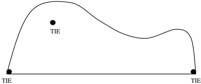
**SET UP INSTRUCTIONS:** There are 6 tie-down areas, 3 on each side. Long straps are for middle tie down and short straps on the ends.
