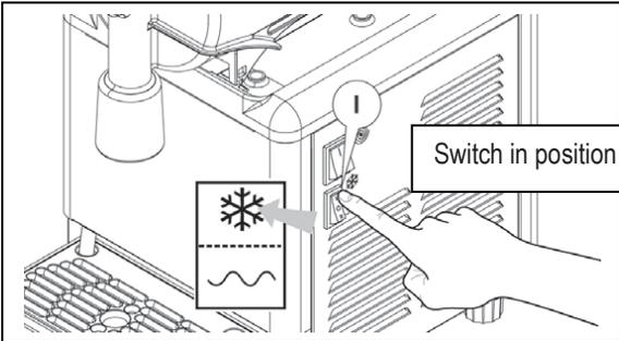
Switch in position "I": refrigeration system on.
